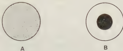
FIG. 260. Illustration of distributional error in absorbance measurements. (A) uniform field, unit area, with 50 per cent transmission, O.D. 0.3, integral of area \times O.D. = 1 \times 0.3 = 0.3 ; (B) same amount of material in 1/100 unit area, O.D. of object 30.0, O.D. of remainder of field 0.0; integral of area \times O.D. = 30 \times 1/100 + 0 \times (99/100) = 0.3 ; however observed transmission = 99 per cent!
